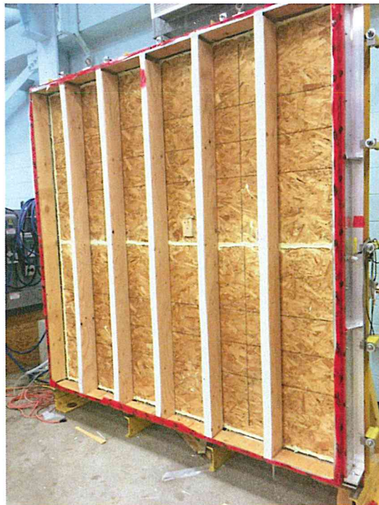
Figure 10: The buckled studs were straightened and reinforced with 3/4in plywood strapping so that the cladding deflection tests could be completed.
